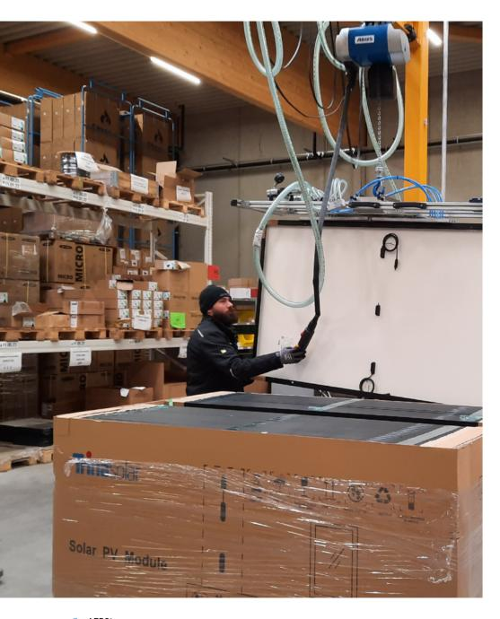
During the manual handling process, at least two people are usually required due to the weight of the individual modules and to protect the material. There is a risk that one of the unwieldy modules could fall down and break. In addition, there is the aspect of ergonomics. Reasons enough to think about optimising this workflow. Due to the neighbouring company locations, the solution was to knock on the door of the vacuum technology professionals next door.
