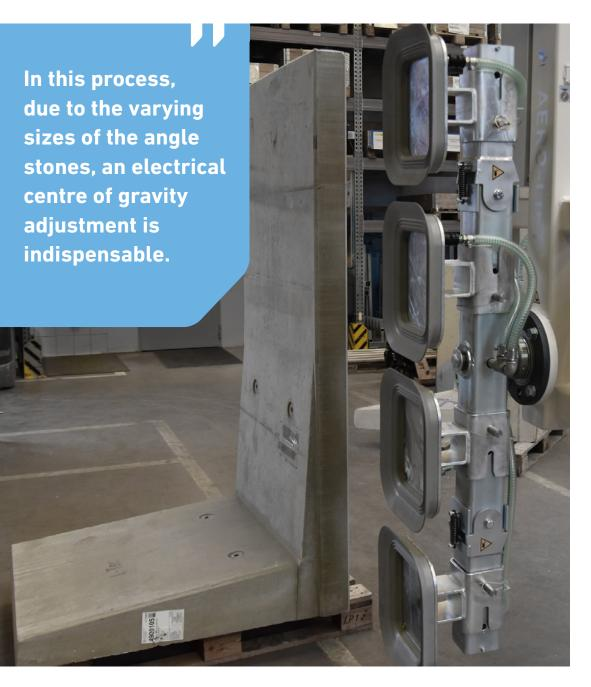
The vacuum lifting device, which was specially developed for the customer, can be operated ergonomically and safely by only one person due to its angled, two-legged manipulation handle. The handle can be flexibly adjusted and locked via a lifting magnet and thus covers an operating angle of 67.5° downwards and 90° upwards.
