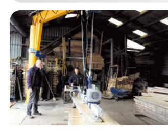
For both types of devices **AERO-TIMBER** and **AERO-PORO** the already existing factory crane can be controlled via the radio remote control of the device.
