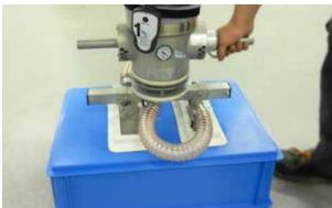
Operating knob in V2A steel design with wireless transmitter
