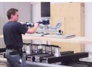
Handling of wooden beams with vacuum gripper suction unit
