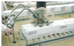
Adjustable operating handle in V2A steel design
