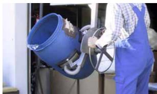
Manual slewing by handwheel
