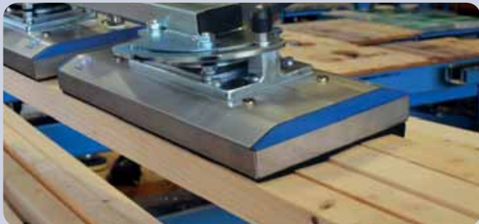
Lifting of individual wooden strips
