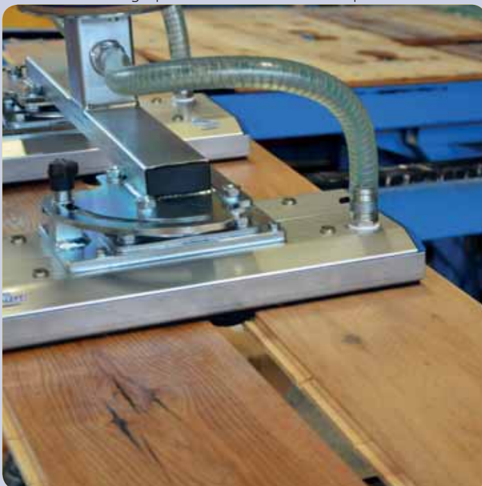
Lifting of wooden flooring segments
