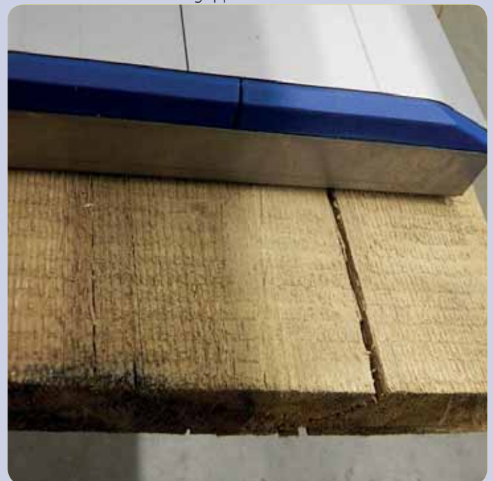
Lifting of wooden boards with cracks or splits
